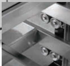
Oversized stainless steel drawer guides
