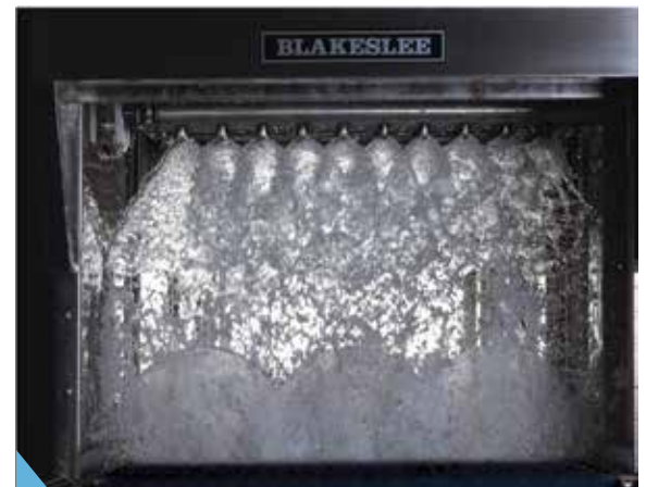
Top and bottom mounted water jets provide torrential cleaning & rinse action.
