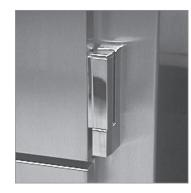
Traulsen uses cam-lift type door hinges. These self-close at up to 90°, have a stay-open feature past 120°, and can be opened past 180° without damage. They are heavy duty and include a lifetime warranty.
