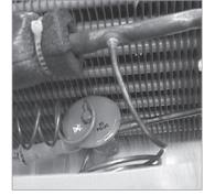
Use of a TXV allows for better temp recovery than possible with capillary tube designs. This is especially important during busy lunch and dinner periods where the doors are opened frequently. Your Traulsen will recover temperature quickly, keeping your food safe and minimizing shrink.
