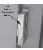
Traulsen solid door models include the light switch concealed inside every door hinge (even on half-height door models). This operates the interior lights automatically whenever the door is opened, while also protecting the switch from damage during loading/unloading.
