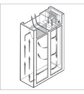
Traulsen's clockwise air-flow pattern keeps cold air in and warm air out much better than back to front designs, which tend to spill cold air out on to the floor whenever opened. A key element is our rear biased return air-duct that protects the system from ingesting warm kitchen air whenever the door is opened.
