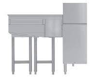
An accessory which adapts to any CLeN that automatically discharges the racks at a 90° angle from the operation of the machine onto a clean table. The DDU38*e* is driven by the conveyor drive of the CLeN and does not require an additional electrical source. The DDU38*e* only adds 38" to the overall length of the machine, but it can save nearly 20 square feet of floor in your dishroom. Stainless steel construction with a 11/2" drain fitting.
