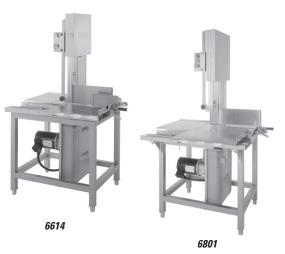
Rigid, open construction with easy to clean, heavy duty carriage support. Stainless steel carriage and table working surface. Stainless steel gauge plate. Bright tinned cast iron upper and lower blade pulleys. Eye-level "On-Off" switch. Positive lock, quick release gauge plate. No tools are needed for removal of parts for cleaning. Designed for complete hose-down,.
