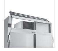
Cleaning the condenser coil is the single most important thing you can do to keep your refrigeration equipment operating efficiently. Traulsen locates this right behind the lift-up louver panel, facing front, making it so easy to clean this can be done in as little as a minute.
