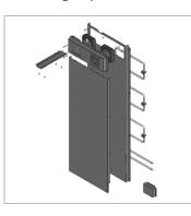
By using large, low watt-density heating elements combined with low velocity fans, Traulsen's hot food holding cabinets offer outstanding performance with no temperature stratification, are ENERGY STAR® certified for efficiency, start-up quickly and greatly reduce lifetime service costs.
